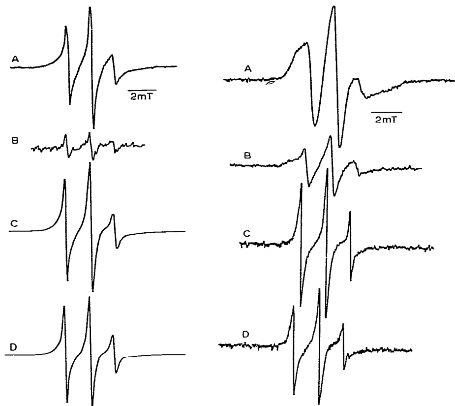
Fig. 1 (left). E.p.r. spectra of glycoproteins treated with spin-label and coupling reagent: A, BSM; B, asialo-BSM; C, fetuin; D, asialo-fetuin.
